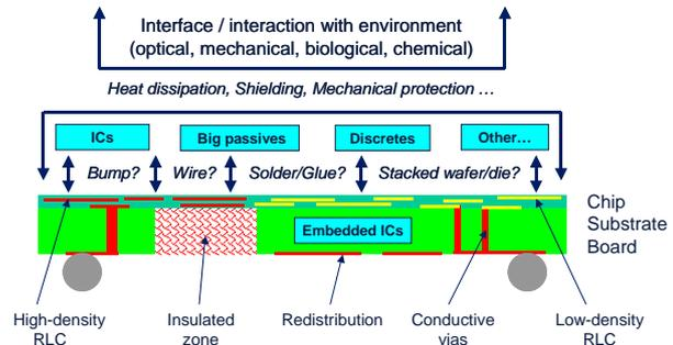
*Heterogeneous integration (SiP) puts multiple technologies into ultra-small packages*
