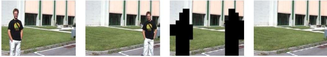
Figure 4. Background recovery from two frames. From left to right: Original frames, background after step 5, output of the algorithm.
