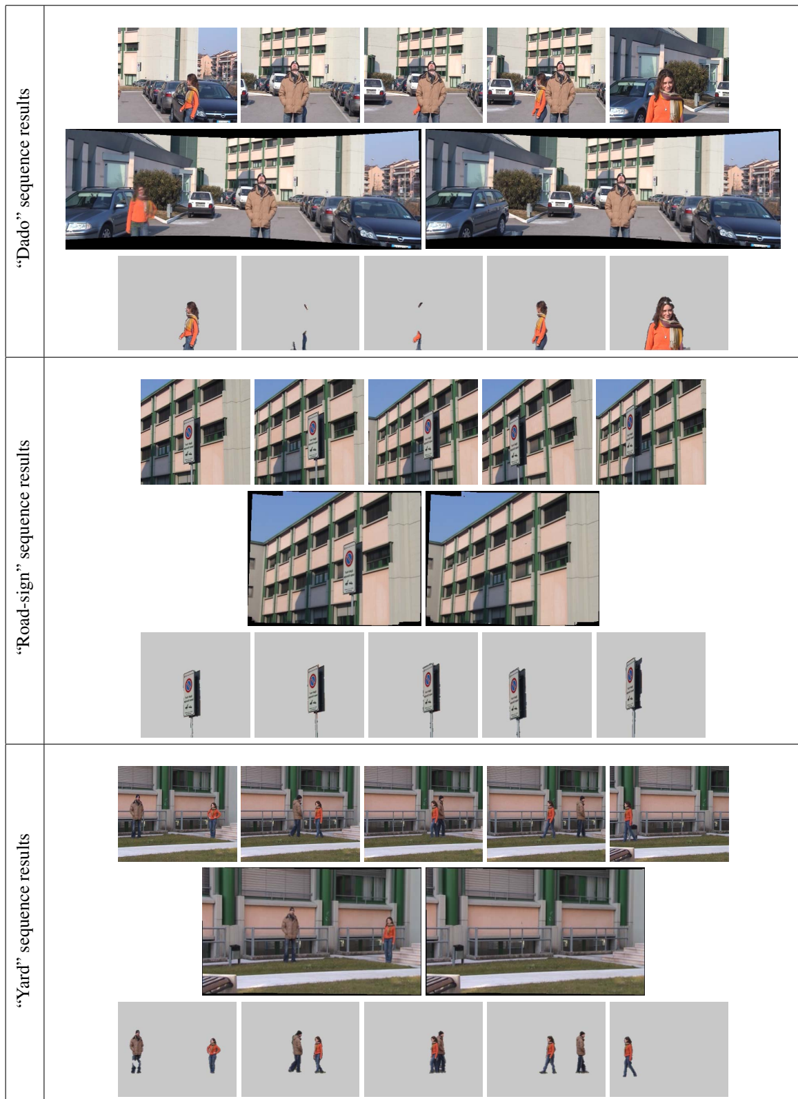
Figure 8. For each sequence, the top row shows some selected frames, the middle row shows the mosaic of the motion-compensated background obtained using the median operator (left) and our technique (right), and the bottom row shows some selected frames of the Video Object sequence.
